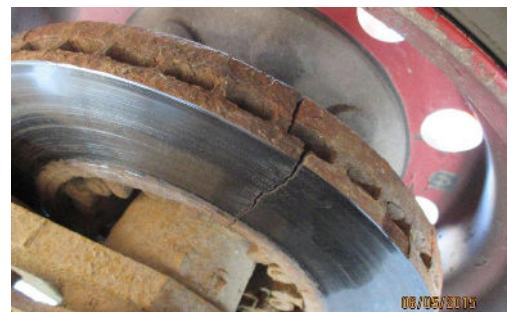
Cracked Rotor. OOSC, Part II, g.(2) / 393.47(a)-U.S.
